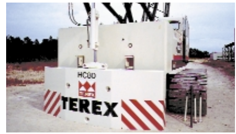
Hydraulic removable counterweight system
