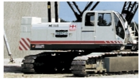
Hydraulic removable counterweight system
